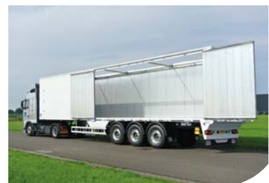
Self-supporting construction with side door opening of 6.8m
